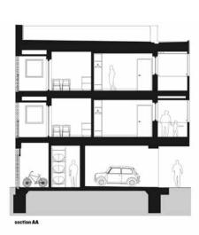
Section showing a integrated parking within the block
